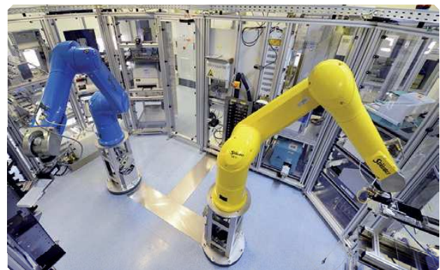
MTS-Roboter (Medium Throughput Screening-Roboter)
